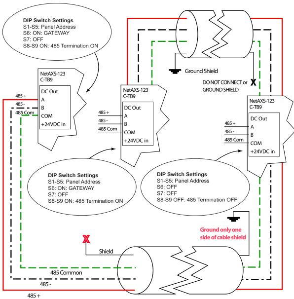
4,000 ft. (1,200 m) max, 24 AWG, 2 twisted pairs with shield, 120 ohm, 23 pf (HAS part no. NCP2441-TN)
